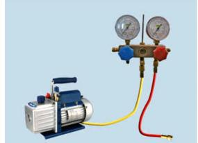
A vacuum pump and maniflod gauge are needed.
